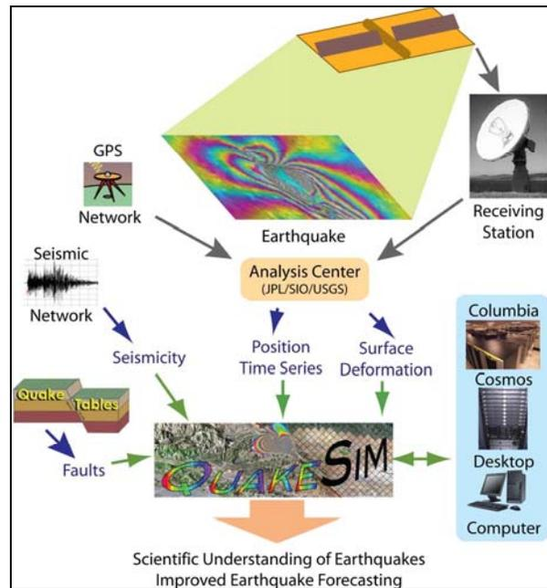
Figure 1. QuakeSim Architecture
