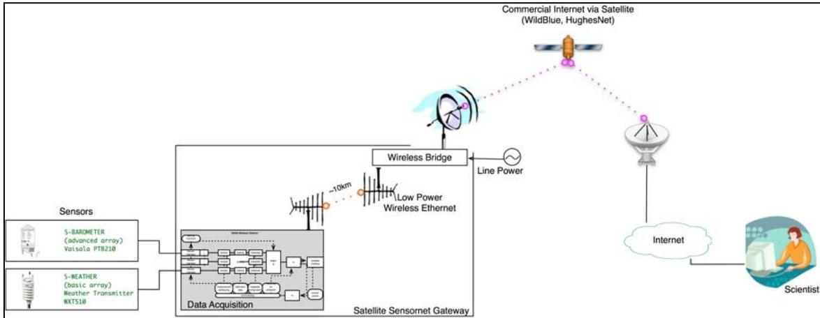
**Figure 5. Satellite Sensor Gateway (SSG)**
